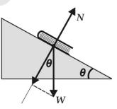
Therefore, if a book is kept on an inclined surface, then the direction of the normal force exerted by the surface on the book will be at an angle that will be perpendicular to the inclined surface.
