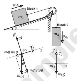
(We have already seen that the magnitude of the tension in the string on both sides of a pulley is the same, and the magnitude of the acceleration of both the blocks is also the same.  $\therefore T_1 = T_2 = T$ , and  $a_{1x} = a_{2y} = a$ ).
