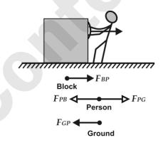
To pull the block, the person has to push forward on the ground with his legs with **action force** of  $F_{GP}$ . Therefore, **reaction force**  $F_{PG}$  of the ground acts on the person to push the person backward. The figure shows two action-reaction pairs as follows. (*Let us assume X-axis to be horizontal with its positive direction on the right-hand side*).
