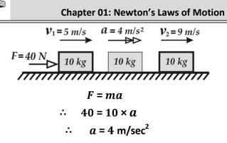
Hence the acceleration of the object will be equal to 4 m/sec<sup>2</sup>. We observe that, as we increased the force to twice the original value, the acceleration also increased twofold in the direction of motion.
