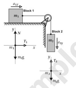
Block 1 is acted on by tension force  $T_1$  in the horizontal direction. The net force  $\sum F_x$  acting on block 1 in the X-axis is as follows.
