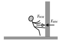
Let us take an example of a man kicking a rigid wall in 'Bruce Lee' style fast-flying kick. As soon as the man applies a force  $F_{WM}$  on the wall by hitting it with a flying kick, the wall produces an equal and opposite force  $F_{MW}$  instantaneously on the man. That is why that man experiences a force that tries to throw him away from the wall. This can be explained as per Newton's third law, which states that for every **action** there is an equal and opposite **reaction**.
