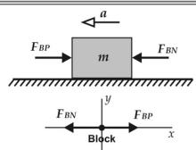
The components of the net force  $\sum F_{\chi}$  acting on the block in X-axis are as follows.
