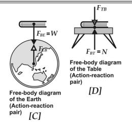
It may be observed that action-reaction pairs of Newton's third law never act on the same object. Therefore, the forces N and W acting on the book are not an actionreaction pair).
