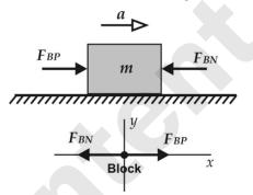
The components of the net force  $\sum F_x$  acting on the block in X-axis are as follows.
